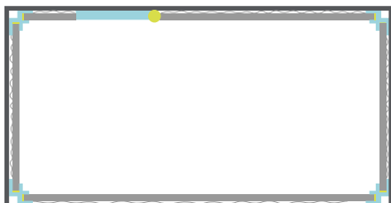
9. Silicone to top of doorway only, then cut panel for above door.
