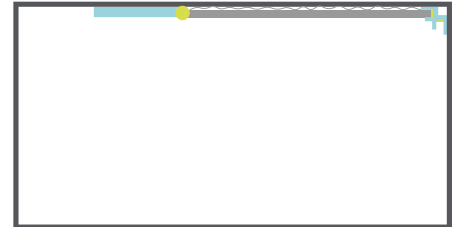
2. Silicone to top of doorway only then continue round room.
