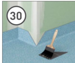
30 Use offcuts to fill in external corners, use heat to soften the vinyl so that it is easy to form tightly around the corner.
